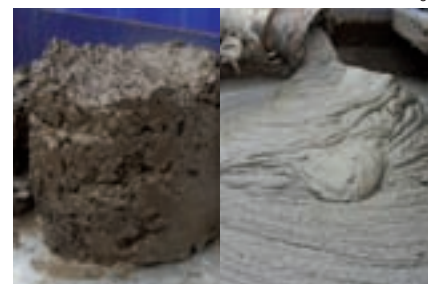
Drill cuttings after shale shaker and after pumping
