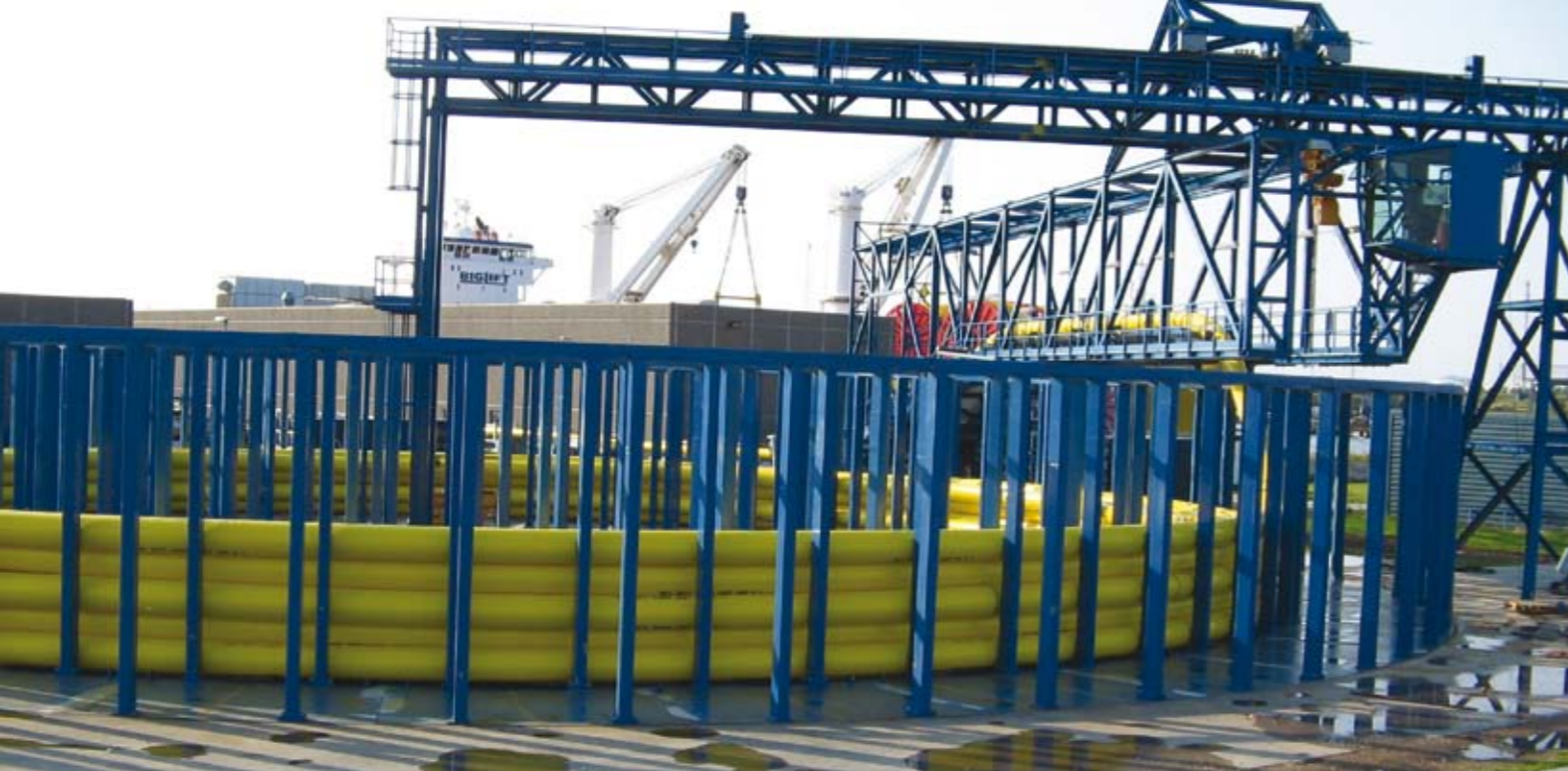
NKT 6000 tonnes carousel. The outer diameter is 41 meter and the height is 4.6 meter.
