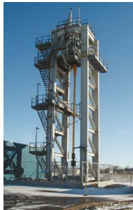
Dynamic fatigue test rig at plant in Kalundborg.
