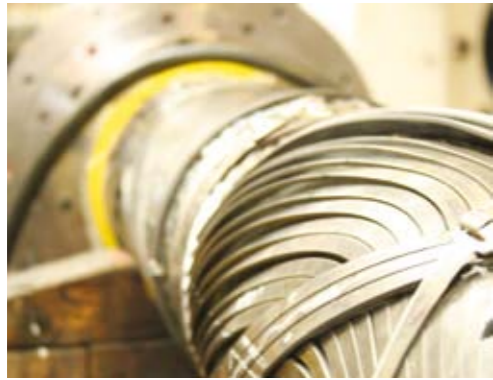
Lateral buckling test in NKT R&D test facilities.
