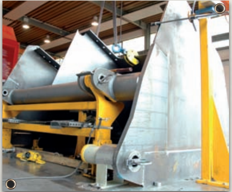
Manufacturing of grab scoops with a size of 12m 3 in a welding jig
