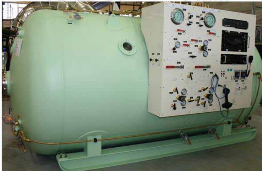
Picture 1. Mix Gas/Air Dive Chamber
