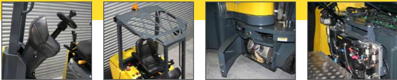
Adjustable Steering Column 4 Post Overhead Guard 19.5kW AC Motor Ease of Access
