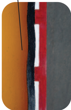
Section through swaged test specimen
