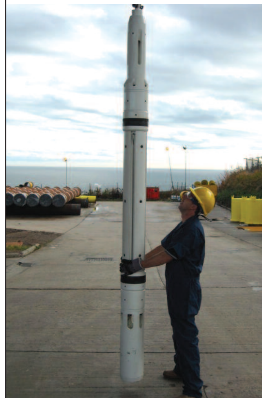
10 3/4" downhole pressure testing tool
