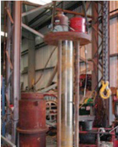
Combined axial internal pressure testing 9 7/8" T95 casing connection
