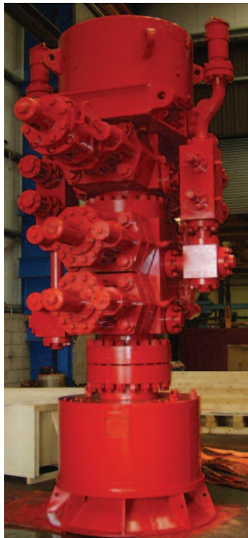
Surface BOP stack
