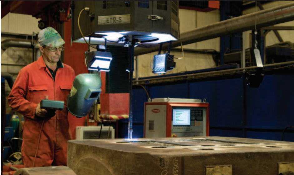
Fronius orbital automated welding system
